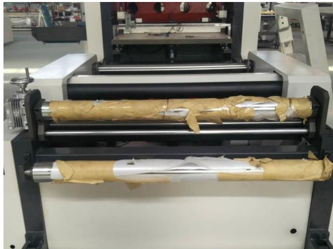
13. Feed material: the photoelectric eye tracking system assures the synchronization of material feeding and die-cutting speed.
