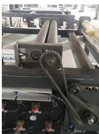
12. Automatically fold and flatten the cornering materials at the paper core. It realized the multistage adjustment of the folding degree. No matter how bent the product is, it can be flatten or refolded towards other directions.
