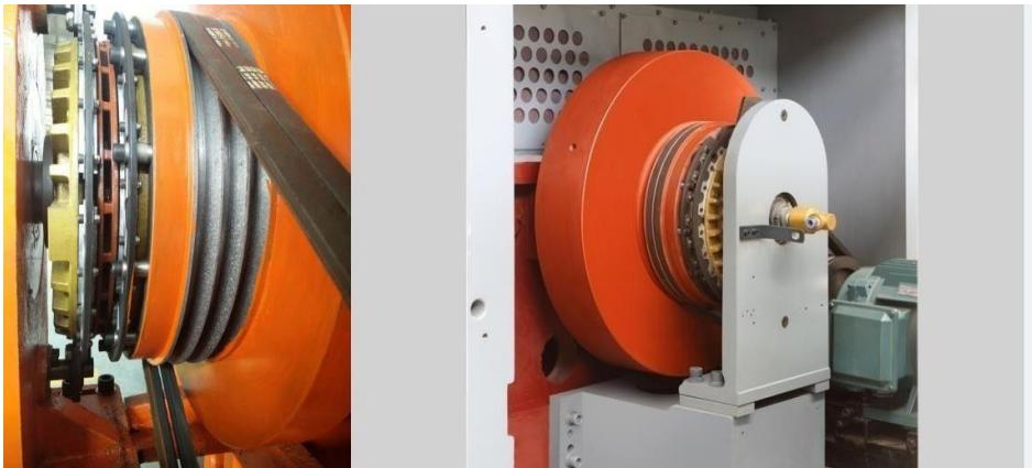
4. Electrical control pressure: accurate and fast to achieve die-cutting pressure adjustment, The pressure is automatic adjusted through the motor to control the four feet by HMI. It is very convenient and accurate.
