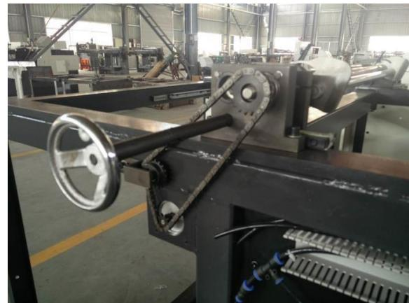
8. Die cutting department adopts pneumatic lock version of the device to avoid coming off from the machine. Die cutting plate: 65Mn steel plate heating treatment, high hardness and flatness.
