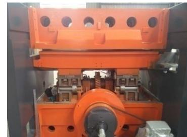
2. Lubrication System: Adopts forced lubrication system to ensure main driving oil supply regularly and reduce friction and prolong the machine life, machine will shut down for protection if oil pressure is low. The oil circuit adds a filter to clear the oil and a flow switch to monitor lacking oil.
