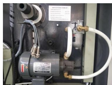
3. The die-cutting force is provided by a 7.5KW inverter motor driver. It is not only power-saving, but also can realize the stepless speed adjustment, especially when coordinate with the extra large flywheel, which make the die-cutting force strong and steady, and the electricity can be further reduced.
