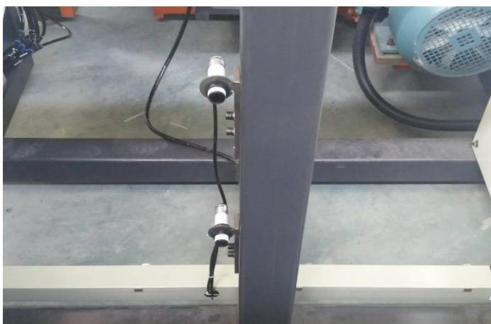
14. By the action of the entity induction switch, finished product will be automatically lowered down to remain the height of the piling paper unchanged, during the whole die-cutting process, manual paper-taking is not needed.
